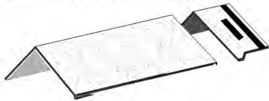
Figure 23 - Cutting an EZ-Ridge™ Shingle to Make a Hip and Ridge Starter Shingle
