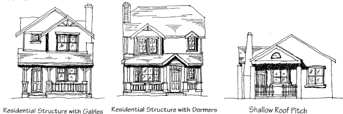
Figure 4-10. Variable rooflines, entries, and porches.
