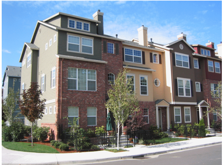
Figure 3-39. This building uses brick for more than 10% of the façade, a decorative mix of materials and colors, decorative entries, and decorative windows to add visual interest.
