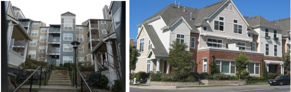
Figure 3-34. This multifamily building uses a combination of horizontal and vertical modulation, roofline modulation, distinctive window patterns, and clear articulation of the building's top, middle, and bottom to help reduce its perceived architectural scale and add visual interest.
