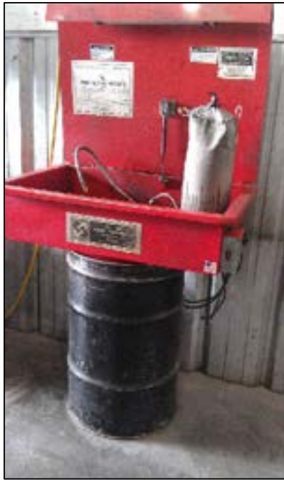
Photograph 35: One of two mineral spirits parts washers in Building B.
