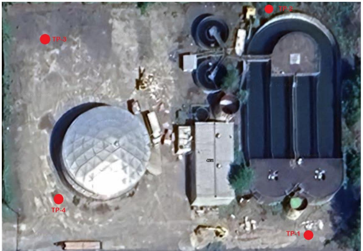
Figure 1 -Approximate locations of test pit excavations and standpipe installations.
